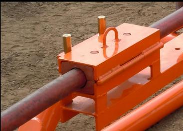
The F14W-XX Strain Relief Clamps are steel manufactured with a variety of available replaceable polyurethane liners sized specifically to fit your cable diameter. The clamp is designed for permanent fixture on shovel stingers, draglines, drills and substations where a fixed (welded or bolted) clamp is required.
