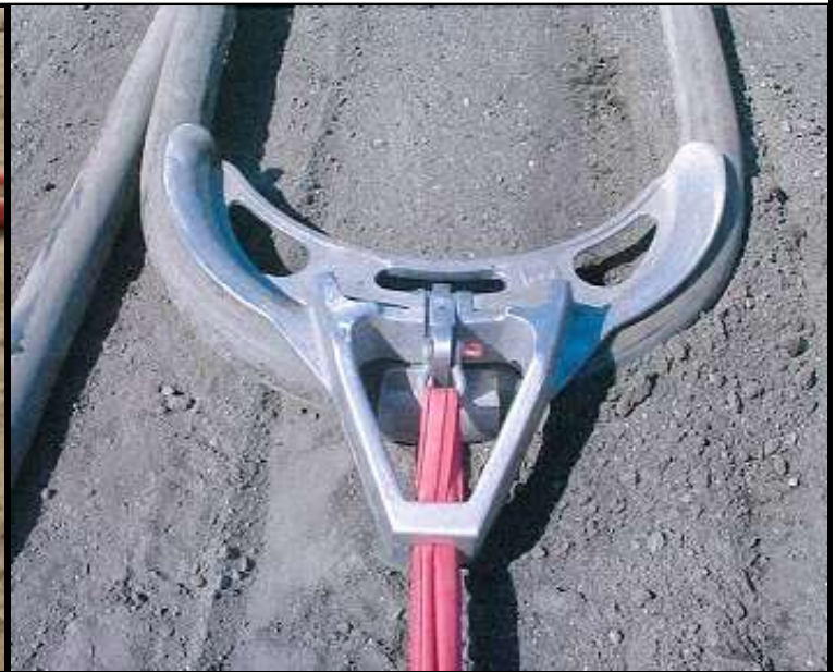
Shown Above: Cable Handling Grab designed specifically for properly cradling cable during trailing cable relocation
