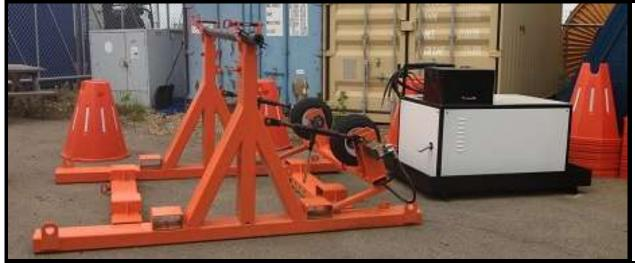
Dual Rim Drive Cable Reeler with variable speed hydraulic power pack.
