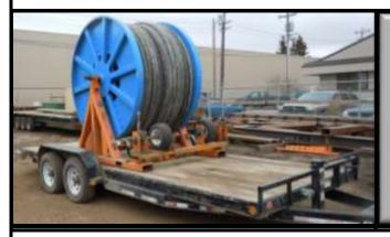
This unit is also our standard rental unit model. Each rental includes the reeler frame, hydraulic power pack, and one certified spindle for your specific requirements.
